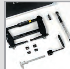
SG6TM KIT (SG6TMSTD) Includes Collets: M24 (7/8") M27 (1")
